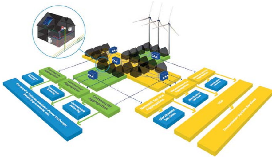
Figure 6: Orthogonal dual market-based architecture for agent-based multi-stakeholder optimization in future electricity systems.
